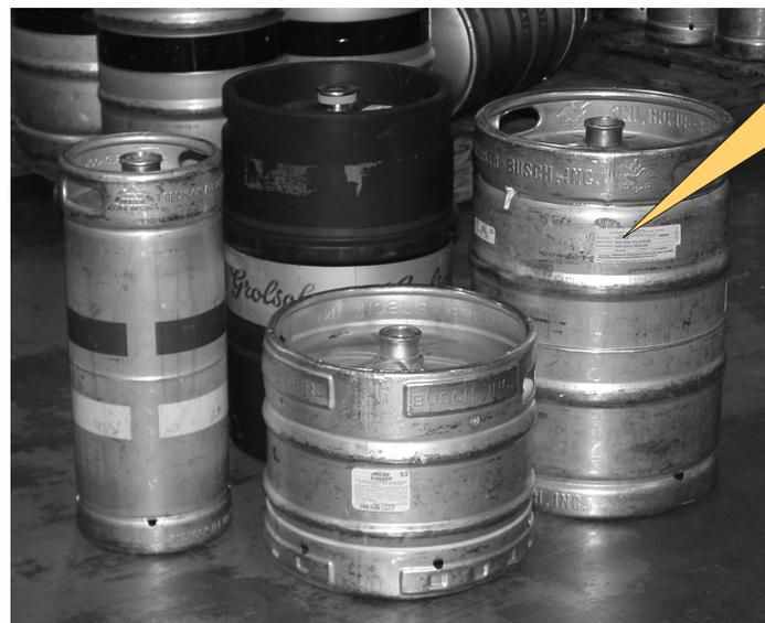
**BY THE GALLON:** Keg beer is sold in various sized containers (clockwise from the right) half barrel (15.5 gallons), one-quarter barrel (7.75 gallons), sixth barrel (5 gallons), and import keg (13.2 gallons). Beer Keg Registration Tag (right) identifies origin of keg and contains an ABC identification tag number that can also be used to trace the origin of the product.
